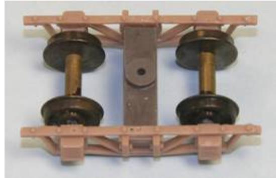
**Step 3:** (Center & right photo) Insert the wheels and hold in place with X-Acto® knife handles or similar. Drop the bolster over the pins. There should be no side-to-side “slop” between the bolster and pin retainer ring, only enough to allow rotation around the pin. Press the ring closer to the back of the sideframe to tighten the fit and test again. Once satisfied, put a small drop of CA on the pin to lock the ring in place.
