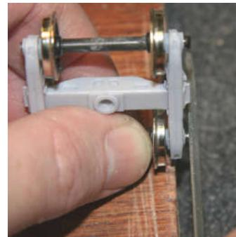
**Step 5:** (Photo at far-right) Axles are intentionally a little long to accommodate manufacturing tolerances and tapering required to align wheel on tube. Once the truck is assembled, you can remove **some** of the axle extension by pressing the wheelset against the sideframe and gently filing off a little at a time, testing often. Be sure the filed axle end is parallel to the sideframe "bearing" or the end cap will wobble.
