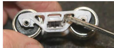
**Step 3:** (Lower-right photo) Pick up a spring using VERY sharp tweezers with smooth jaws. Place over the middle boss in the 2<sup>nd</sup> row of the sideframe, compress it slightly, then align over the matching center boss in the bolster. Repeat for all springs across the front (2 or 3). No glue is required to hold springs in place. Repeat for the other side of the truck.
