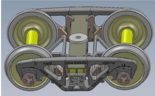
(Left) >> a Solidworks 3D CAD screen shot of an assembled Barber 50-ton roller bearing truck with 33" wheels, triangular rotating end caps and brake shoes/beams.
