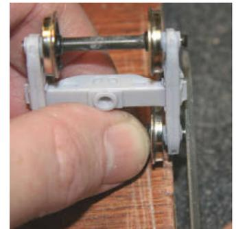
**Step 5:** (Photo at far-right) Axles are intentionally a little long to accommodate manufacturing tolerances and tapering required to center wheel on tube. Once the truck is assembled, you can remove some of the axle extension by pressing the wheelset against the sideframe and gently filing off a little at a time, testing often. Be sure the filed axle end is parallel to the sideframe "bearing" or the end cap will wobble.
